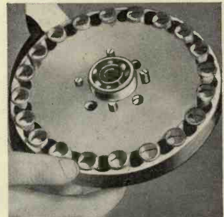
Fig. 1. The transmitter scanning disc is of the lensed type.
