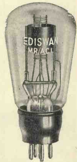
The Ediswan mercury-vapour relay used in the synchroniser.
