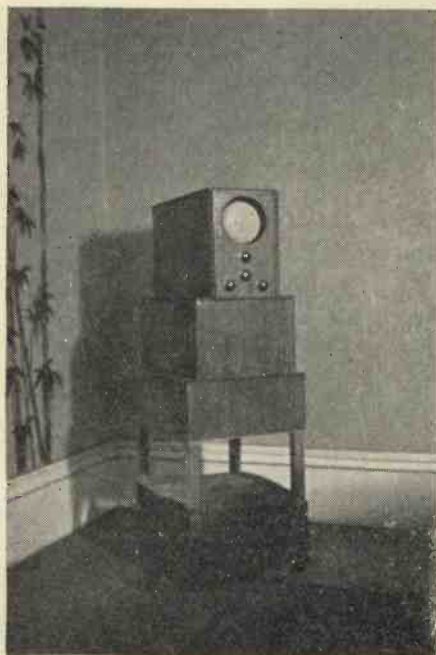
The Gillavision cathode-ray receiver is entirely self-contained.
